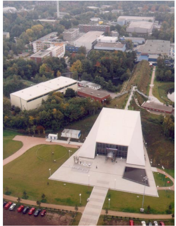
Fig. 5. Aerial view of the experimental hall for the FEL User Facility (front, center) and the tunnel for the TTF phase 2 extension behind it (covered with grass). The hall in the upper right corner houses the TTF phase 1 FEL.
